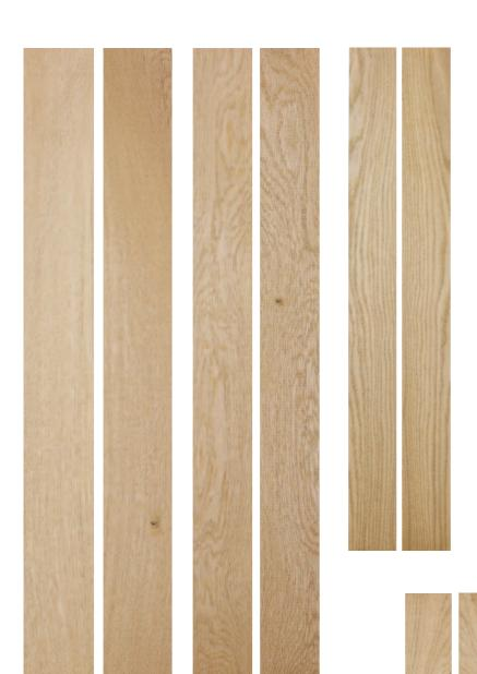
For all grades, the letter X indicates the presence of sound sapwood less than two thirds of the thickness, and XX if it is present on both faces.
